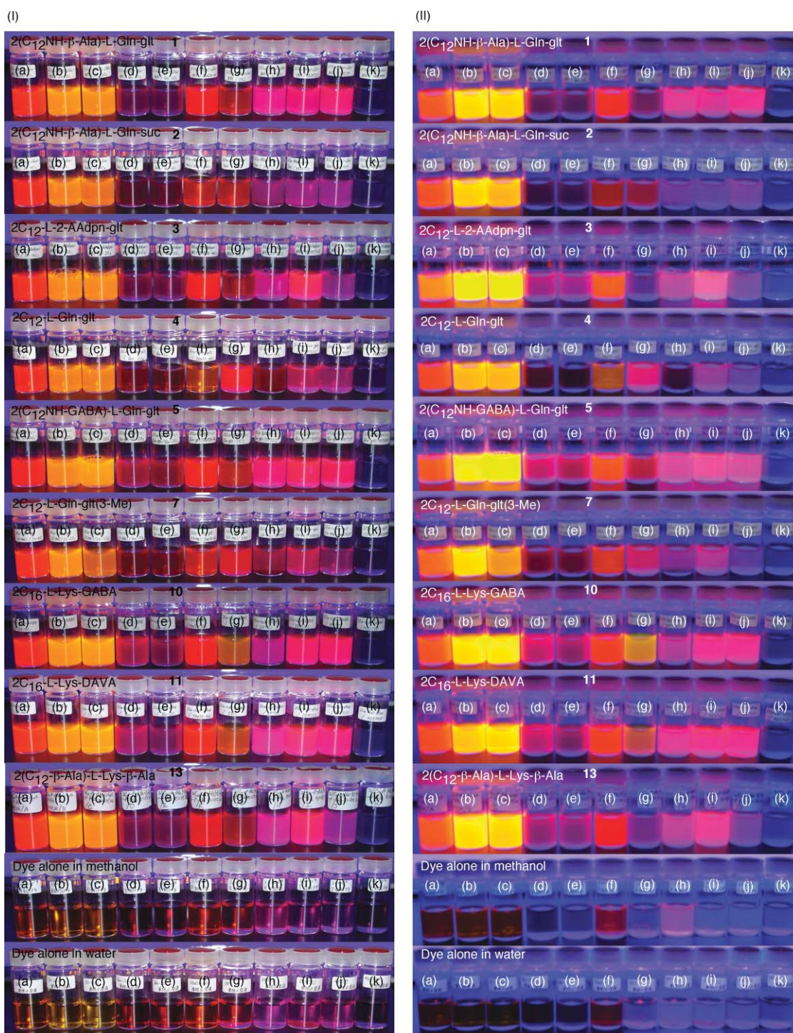
Fig. 2 Photographs of aqueous cationic dyes in the presence of various anionic peptide amphiphiles in water; [amphiphile] = 3.0 mM, [dye] = 0.15 mM, pH 10, 20 °C. (I) under black light irradiation in the daytime. (II) under black light irradiation in the dark. The abbreviations of dyes used in this study are as follows: (a) St-4C 1 , (b) St-2C 1 , (c) St-2C 2 , (d) Qu-2C 2 (Quinaldine Red), (e) Qu-2C 1 , (f) DBASt-4C 1 , (g) DEC, (h) DPTCC, (i) DE9MTCC, (j) DE9ETCC (NK-737), and (k) MDEPAP.
